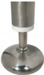
Part. R0752 - Pag. R44 Ø 120 • Stainless steel • Hygiene • Max. load 12000 N.
