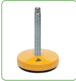
Part. R0403 - Pag. R50 Ø 100 • Painted steel • Max. load 50000 N.
