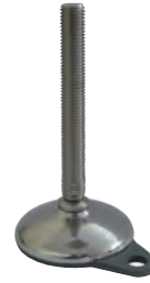
Part. R0748F - Pag. R43 Ø 100 • Stainless steel • Hygiene • Prefitting for fixing • Max. load 25000 N.
